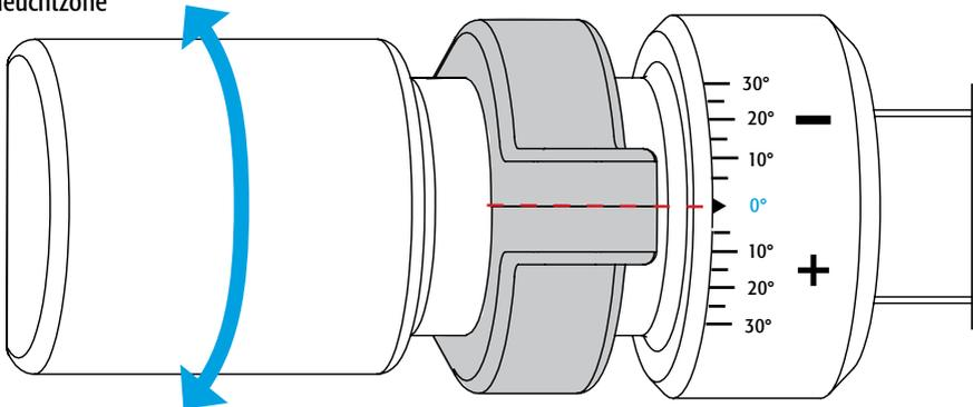
Align Skew angle indication with arrow point or split line (highlighted in red).
