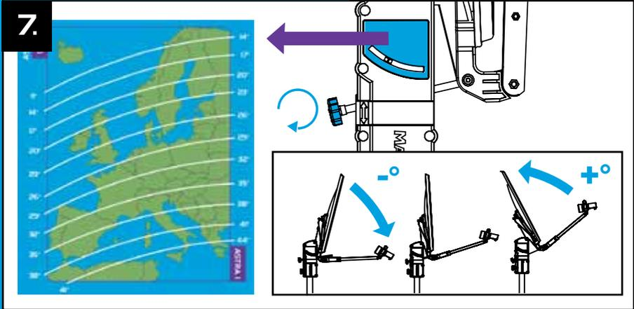
7. Use the elevation map to determine the required angle for your location.
