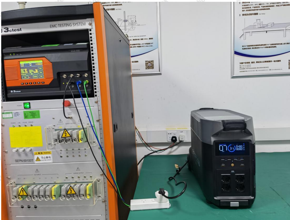
Photo of Surge Test
