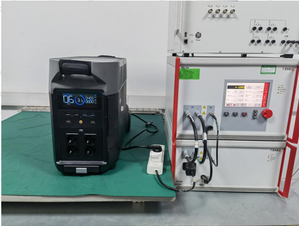
Photo of Electrical Fast Transient /Burst Immunity Test
